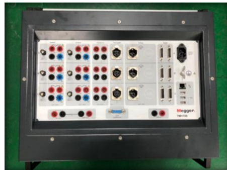
Circuit Breaker Analyzer
