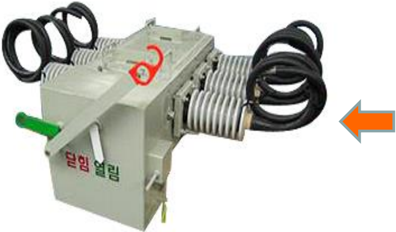
SF 6 Gas ASS 25.8kV, 400A 12.5kA, 60Hz
