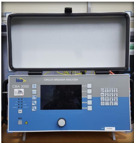
Circuit Breaker Analyzer
