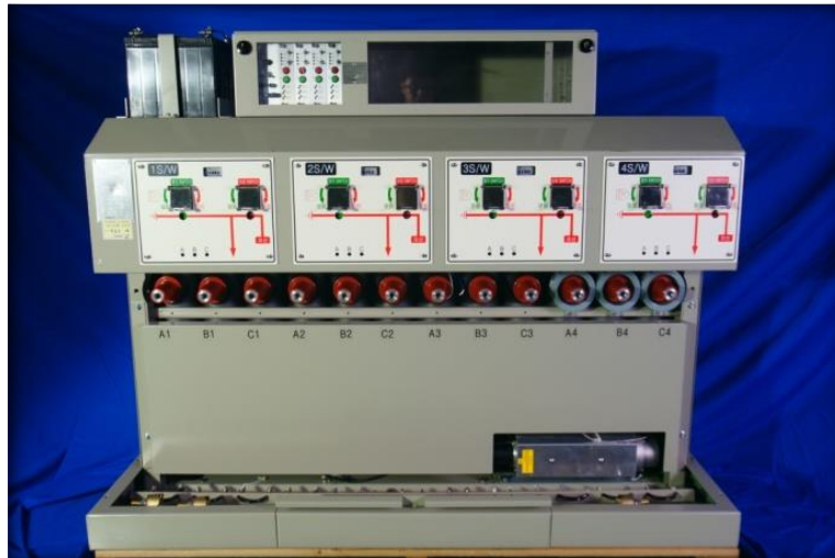
Epoxy Mold LBS (Underground) 25.8kV, 600A, 12.5kA, 60Hz 3~4 ways
