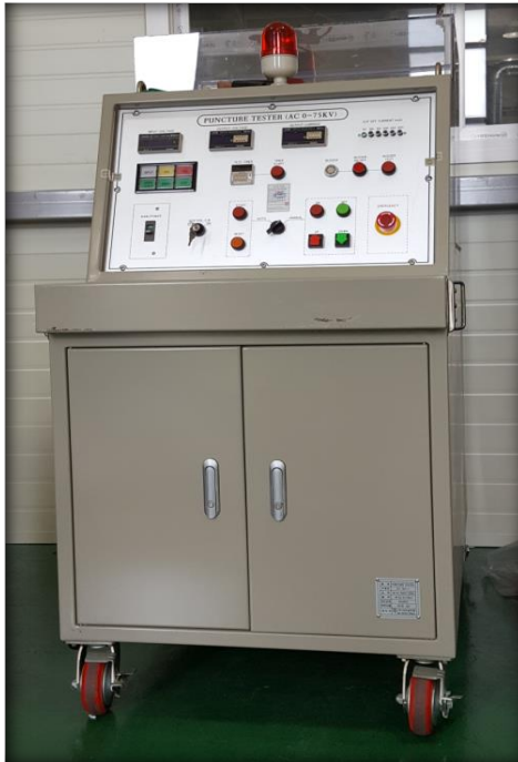
Voltage Withstand (75kV 300mA 22.5kVA)
