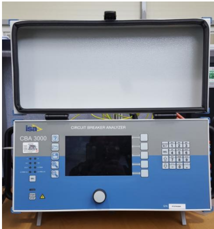
Circuit Breaker Analyzer
