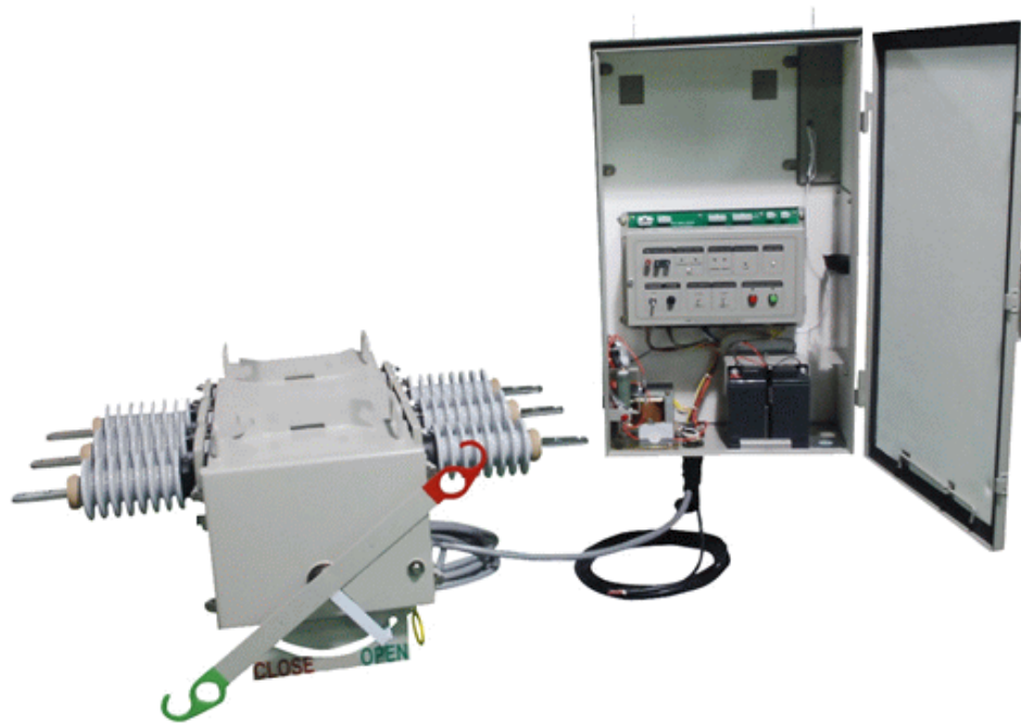
SF 6 Gas LBS : Terminal Type 12~36kV, 400/630A 16kA, 50/60Hz
