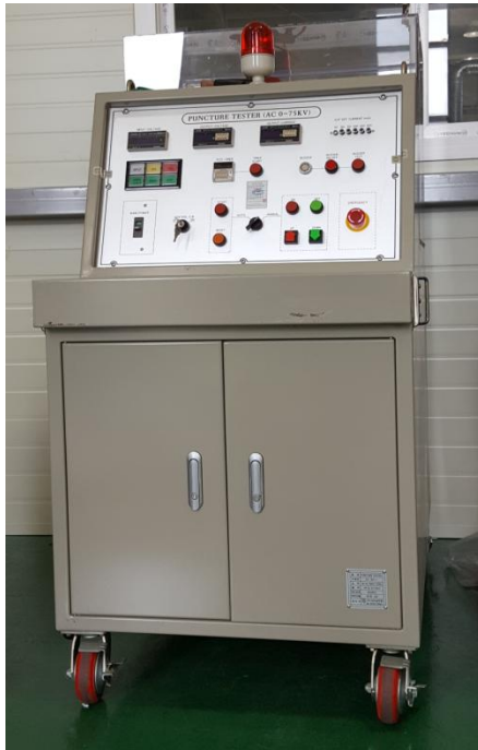
Voltage Withstand (75kV 300mA 22.5kVA)
