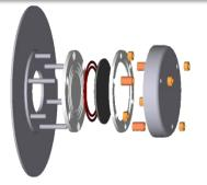
• Relief membrane burst for safty at internal overpressure
